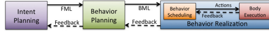
Fig. 2. Our subdivision of SAIBA’s Behavior Realization layer into the Behavior Scheduling and Body Execution sub-layers.
