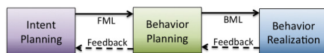
Fig. 1. The three stages of behavior generation in the SAIBA framework and the two mediating languages FML and BML. [9, 6]
