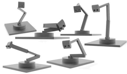
Figure 5: The concept design of the Adelino robot. It was initially modelled and animated using 3D animation software, to explore the size and placement of each segment and articulation, in order to maximize its expressive capabilities. Note that in this image, at some points, there are articulations that can rotate more than 90 degrees to each side. This feature was not maintained in the actual robot due to typical servos’ limitation.
