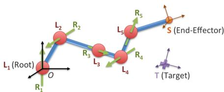
**Figure 1: An articulated structure (kinematic chain) as used in both Forward Kinematics (FK) and Inverse Kinematics (IK). Also shown is a given target T that is to be reached by the end-effector S.**
