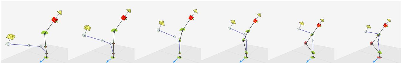
**Figure 8: Demonstration of orientation hold during posture shifts. Two shifts of posture are shown, one for a common easy orientation, and another for a more complicated, extreme orientation. The blue arrow represents the character’s frontal direction. The remaining elements are described in the caption of Figure 7.**
