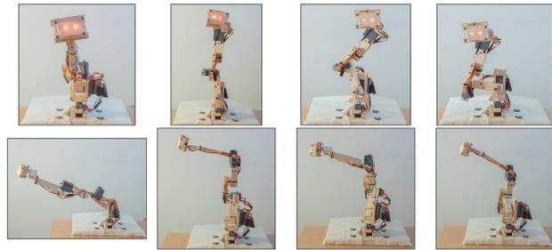
**Figure 6: The Adelino robot, in four different expressive postures. The top row shows front views of each posture. Under each is the corresponding side view.**
