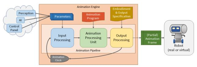
Figure 23: A *Nutty*-based animation engine, including the *Nutty Pipeline*. At each clock cycle, the Input parameters along with the selected Animation Program are provided to the Animation Program Processor, which outputs a (Partial) Animation Frame contains the motion parameters for each programmable DoF.
