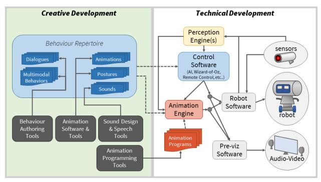
Figure 22: The *Nutty* robot animation workflow.
