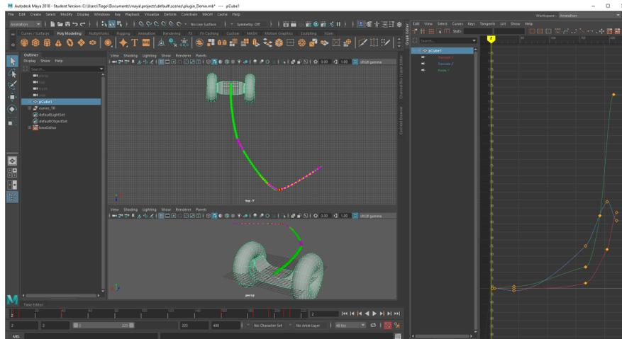
**Fig. 23** A screenshot illustrating the robot-animation trajectory-helper feature implemented through a plug-in into Autodesk Maya. This feature draws the motion trajectory as a path directly into the scene of the animation software, and highlights the points of the trajectory that break any of the robot’s kinematic limits.
