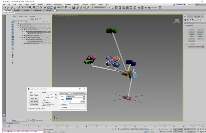
**Fig. 22** A screenshot of the Natty Tracks plug-in for Autodesk 3dsmax, illustrating the skeletal animation rig created by the plug-in. An animator can generate this rig through the simple click of a button, and then use the plug-in to export the final animation to a Nutty-compatible animation file.
