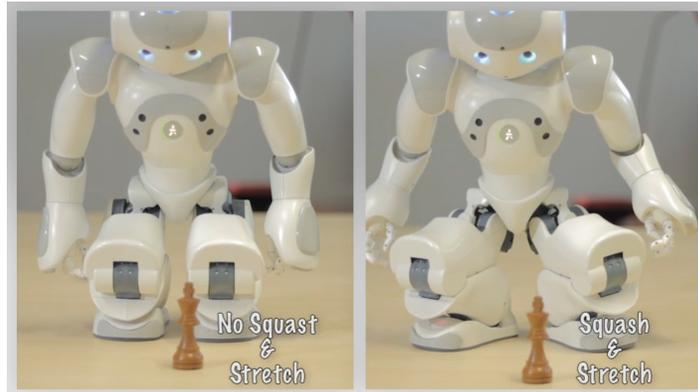
**Fig. 6** The principle of Squash & Stretch shown on the NAO robot.
