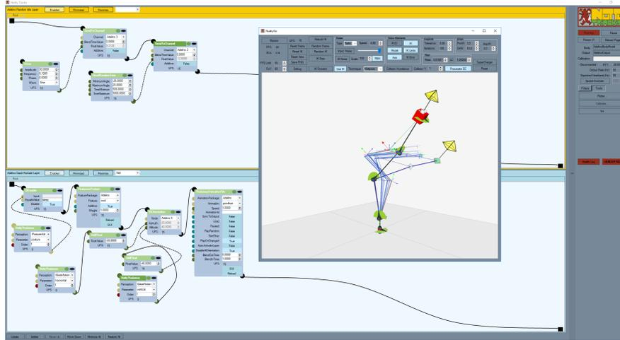
**Fig. 4** The Nutty Tracks standalone GUI, used for composing animation programs, and to execute them in both a virtual window (for diagnostics) and on the real robot.
