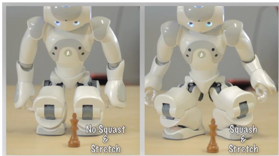
Figure 4.2: The principle of Squash & Stretch shown on the NAO robot.
