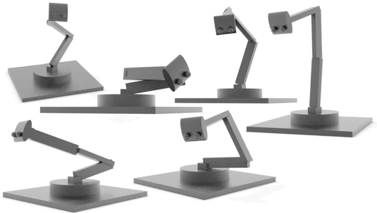
Figure 7.9: The concept design of the Adelino robot. It was initially modelled and animated using 3D animation software, to explore the size and placement of each segment and articulation, in order to maximize its expressive capabilities. Note that in this image, at some points, there are articulations that can rotate more than 90 degrees to each side. This feature was not maintained in the actual robot due to typical servos' limitation.
